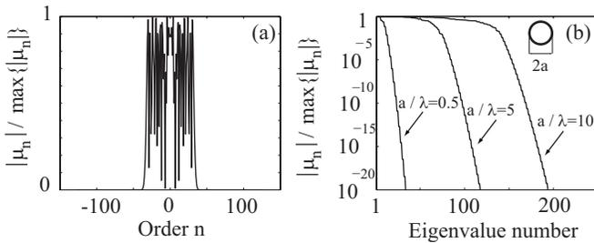
FIG. 3. Eigenvalue structure of the far-field operator calculated for a sound-hard circular cylinder: (a) Normalized eigenvalues corresponding to  $-128 < n < 128$  for  $a/\lambda = 5$ ; (b) eigenvalues reordered from the largest to the lowest for three different radius to wavelength ratios.
