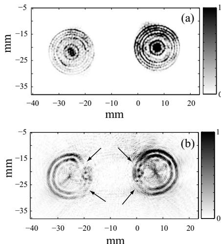
FIG. 16. Monochromatic images of the two rods at 850 kHz ( $\lambda=1.78$  mm). (a) Factorization method; (b) Kirchhoff migration. The arrows in (b) indicate the portions of the rod boundaries which have not been reconstructed.
