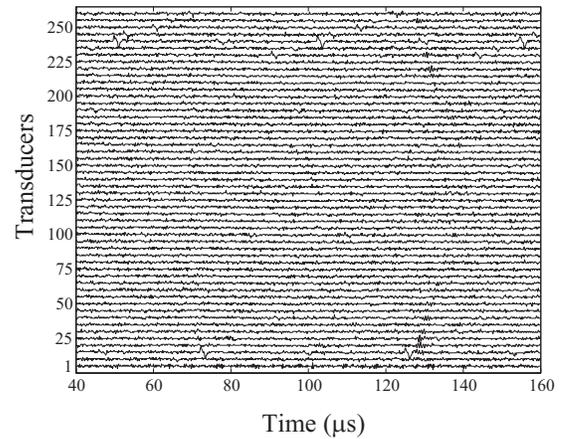
FIG. 9. Pulse-echo time traces measured for the two-nylon-wire experiment. Due to the small size of the wires, the reflected signals which occur between 120–140  $\mu\text{s}$  are weak and buried in the background noise.
