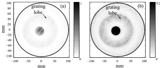
FIG. 6. Monochromatic images of a 34 mm diameter rod obtained with the factorization method at 1.3 MHz ( $\lambda=1.16$  mm): (a) Before threshold; (b) after applying threshold. The dots along the circle represent the actual positions of the array elements.
