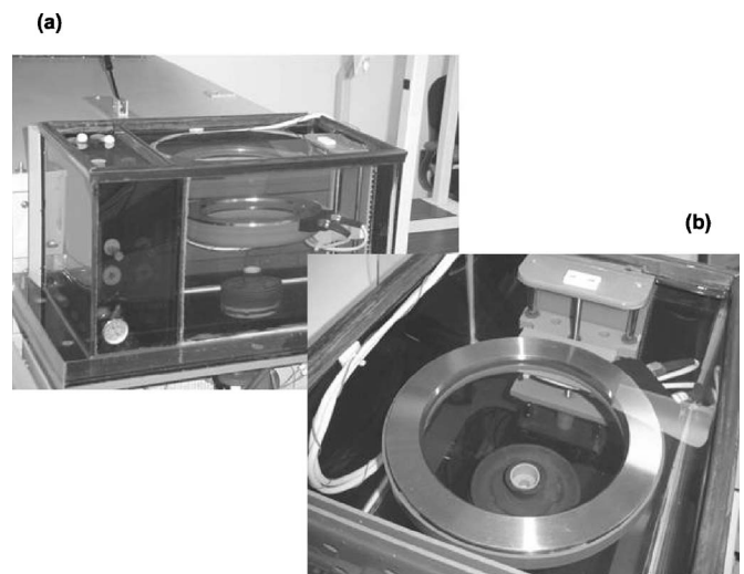
FIG. 5. (a) Imaging tank. The water tank that contains the ring transducer is referred to as the imaging tank. Its temperature is controlled with a heater and is usually set to body temperature. (b) The ring transducer is immersed in water during the scan. It is connected to the electronics under the table via two cables, as shown.
