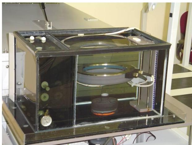
Figure 1. A picture of CURE transducer ring array.
