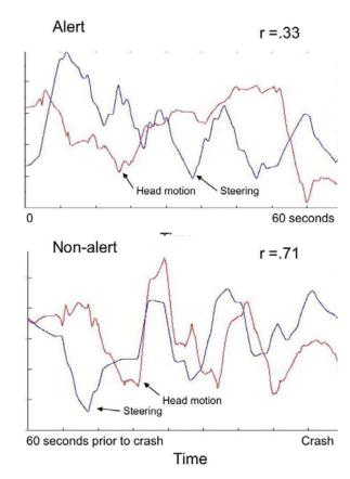
**Fig. 6**. Head motion and steering position for 60 seconds in an alert state (top) and 60 seconds prior to a crash. Head motion is the output of the roll dimension of the accelerometer.
