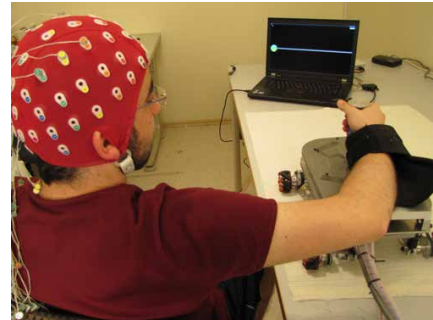
Fig. 1. Experimental setup consisting of the Biosemi ActiveTwo EEG measurement device and ASSISTON-MOBILE
