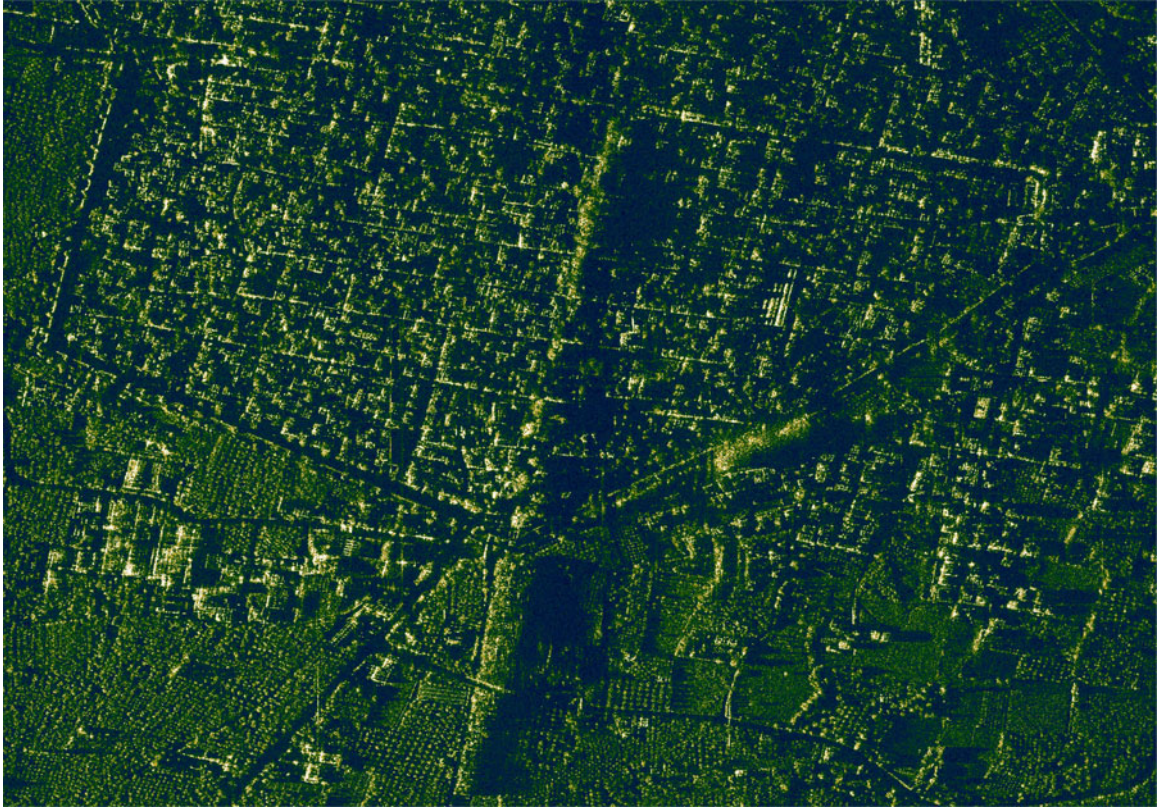
Fig. 10. Reconstruction with the proposed method from 3.2% of reference samples in Fourier space.
