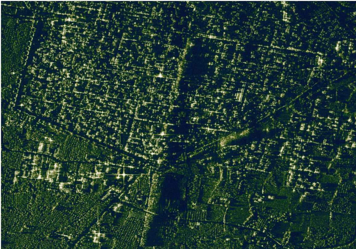
Fig. 9. Minimum-norm reconstruction from 3.2% of reference samples in Fourier space.
