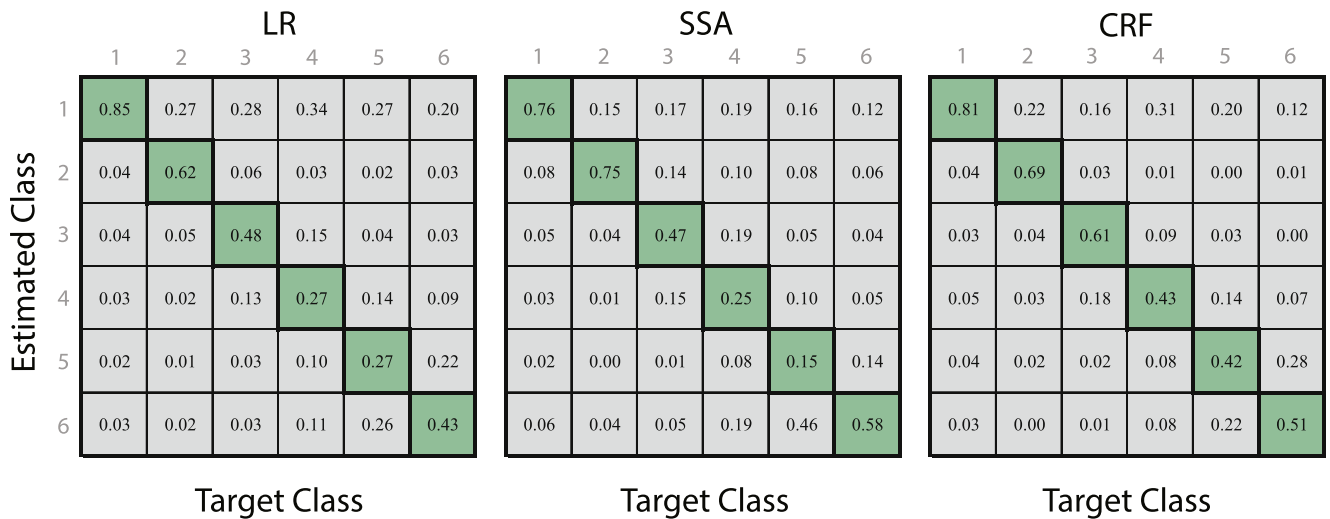
Figure 4. Classification results in terms of accuracy (confusion matrices) for each method across all subjects. Diagonals display the correct classification rate for each class.
