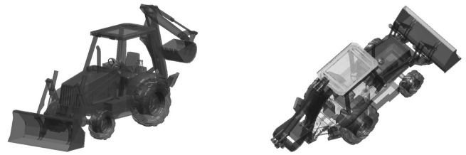
Fig. 8. Backhoe model used in Xpatch scattering predictions. View to right corresponds approximately to view in images in our experiments.
