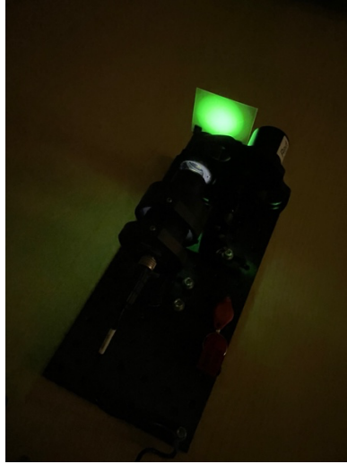
After the white light is turned off, in this case the students will see the phosphorescent paper glow green because blue light has more energy than red or green light and has enough energy to make the phosphorescent paper glow. The glow will fade over time until it completely disappears.
