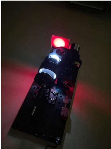
White light shining through the red filter onto the phosphorescent paper.
