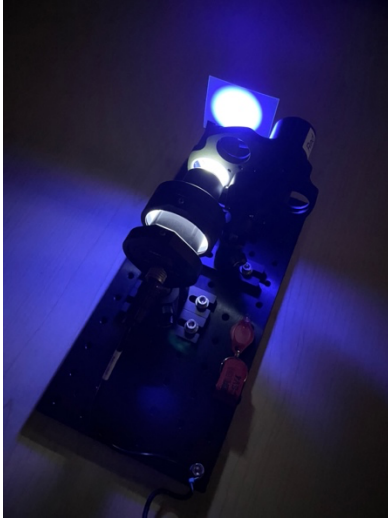
White light shining through the blue filter onto the phosphorescent paper.
