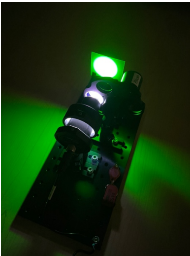
White light shining through the green filter onto the phosphorescent paper.
