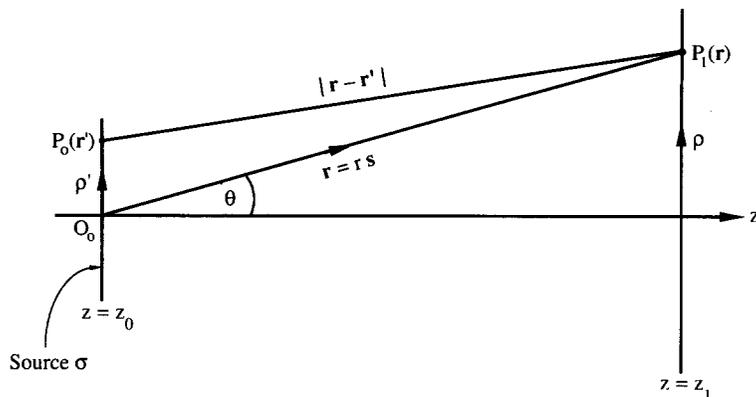
Fig. 2. Illustration of the notation relating to the formulas (8) and (9). The point  $P_1$ , located in the far zone, is specified by the position vector  $r \equiv rs \equiv (z_1, \rho)$ .
