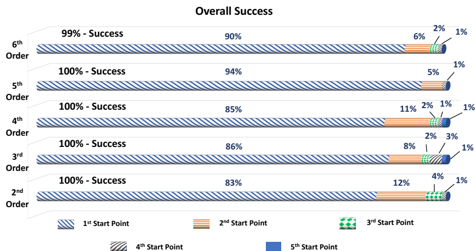
Fig. 5. Percent successful retrievals when three targeted \alpha planes and 5 random starting sets of phase values are permitted (noiseless).
