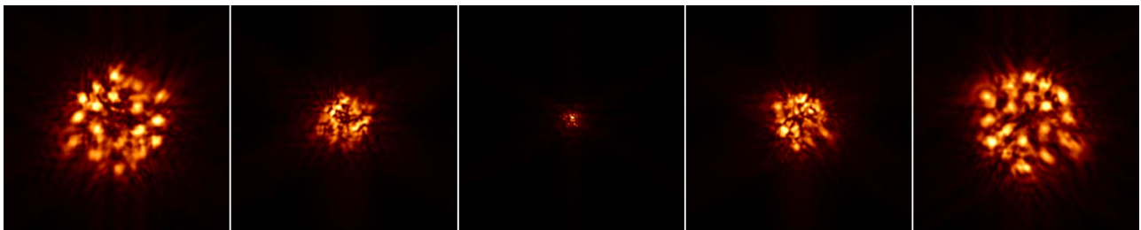
Fig. 5. Sample data PSFs prior to applying noise, with known defocuses of -8\lambda_0 , -4\lambda_0 , 0 , 4\lambda_0 , and 8\lambda_0 from left to right. For these PSFs, the maximum path difference is 3.0\lambda_0 , the global RMS WFE is 0.15\lambda_0 , and the (non-piston) per-segment RMS WFE is 0.05\lambda_0 . Each PSF array has been square-rooted element-wise to show dimmer features.
