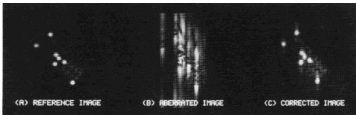
Figure 1. Phase-error correction example. (A) Diffraction-limited image of a synthetic complex-valued object; (B) aberrated image, smeared by 1-D Fourier phase errors in the vertical direction; (C) image obtained from the Fourier transform corrected for phase errors using the shear averaging algorithm.
