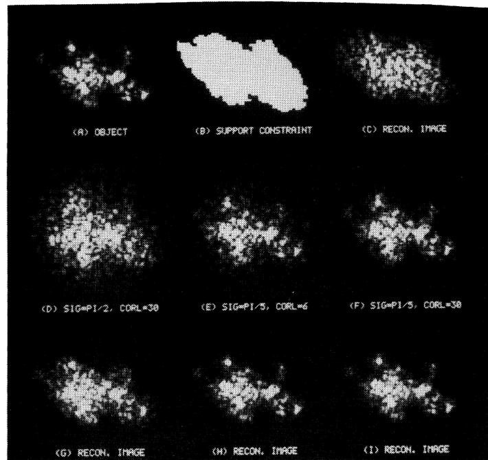
Figure 3. Reconstruction of complex-valued images by the phase variance algorithm. (a) Object; (b) support constraint; (c) image reconstructed with no phase information; (d)-(f) blurred images, with (d) phase errors  $\sigma = \pi/2$  radians and  $\text{corl} = 30$  pixels, with (e)  $\sigma = \pi/5$  and  $\text{corl} = 6$ , and with (f)  $\sigma = \pi/5$  and  $\text{corl} = 30$ ; and (g) - (i) corresponding images reconstructed by the phase variance algorithm.
