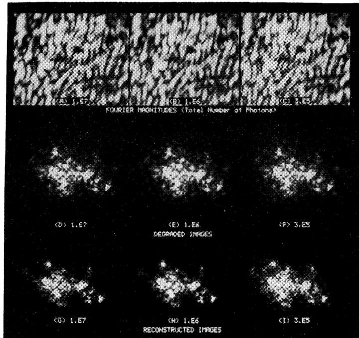
Figure 5. Reconstruction of complex-valued images by the phase variance algorithm with photon noise. (a) - (c) Noisy Fourier modulus estimates (their squares, the intensities, were subjected to photon noise), with (a)  $10^7$ , (b)  $10^6$ , and (c)  $3 \times 10^5$  total photons; (d) - (f) images degraded by the phase error; and (g) - (i) the corresponding reconstructed images.
