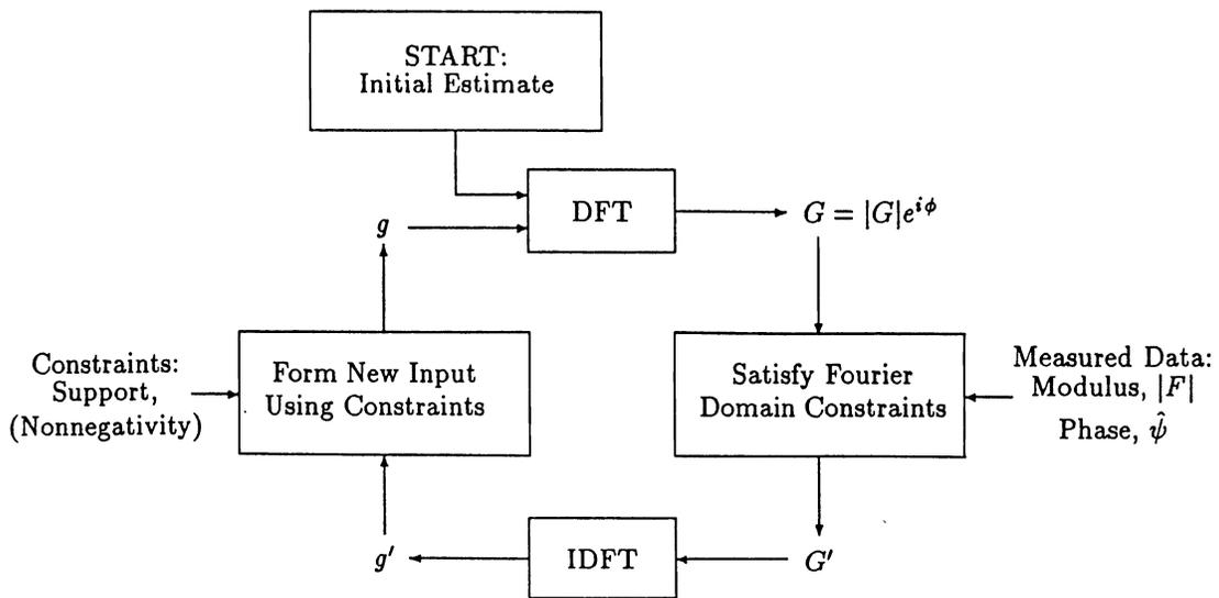
Figure 2. Block diagram of the phase variance version of the iterative transform algorithm.
