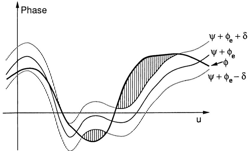
Figure 1. Fourier-domain phase modification by the phase variance algorithm. The phase  $\phi'(u,v)$  is constrained to lie within  $\delta = c\sigma$  of the given phase,  $\theta(u,v) = \psi(u,v) + \phi_e(u,v)$ .
