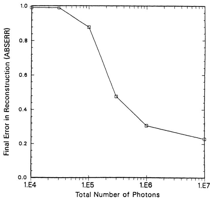
Figure 4. RMS error of the reconstructed images as a function of the total number photons.
