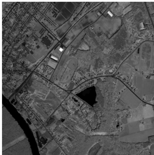
Fig. 2. Panchromatic representation of multi-spectral object. The object consists of 11 spectral bands, centered about 1 μm and spanning 96 nm.
