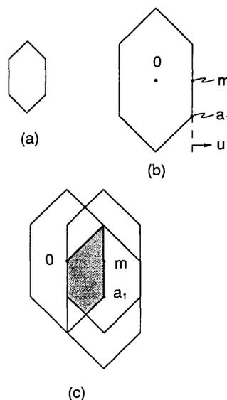
Fig. 9. Example of the  $u$ -convex rule. (a) Set  $S$ ; (b) set  $A = S - S$ , where  $a_1$  and  $m$  are an endpoint and the midpoint, respectively, of  $E(A, u)$ ; (c) a single-sided locator set  $L = A \cap (A + a_1) \cap (A + m)$  determined by the  $u$ -convex rule (indicated by the shaded area).
