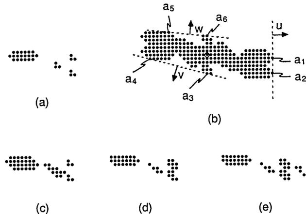
Fig. 5. Example of the two-point rule. (a) Set  $S$  consisting of discrete points; (b) set  $A = S - S$  with  $E(A, u) = \{a_1, a_2\}$ ,  $E(A, v) = \{a_3, a_4\}$ , and  $E(A, w) = \{a_5, a_6\}$ ; (c) single-sided locator set  $L_1 = A \cap (A + a_1) \cap (A + a_2)$ ; (d) single-sided locator set  $L_2 = A \cap (A + a_3) \cap (A + a_4)$ ; (e) single-sided locator set  $L_3 = A \cap (A + a_5) \cap (A + a_6)$ .
