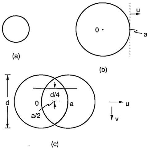
Fig. 11. Example of the one-point rule. (a) Set  $S$ ; (b) set  $A = S - S$  and  $E(A, u) = \{a\}$ ; (c) single-sided locator set  $L = A \cap (A + a) \cap H$ , where  $H$  is determined by the displayed  $u, v$ , and the one-point rule as in Theorem 6.
