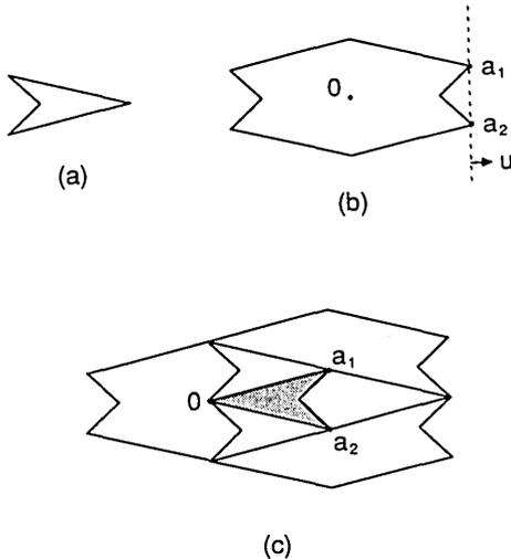
Fig. 4. Example of the two-point rule. (a) Set  $S$ , (b) set  $A = S - S$  and  $E(A, u) = \{a_1, a_2\}$ , (c) shaded area is the single-sided locator set  $L = A \cap (A + a_1) \cap (A + a_2)$ , which is identical to a translation of  $-S$ .
