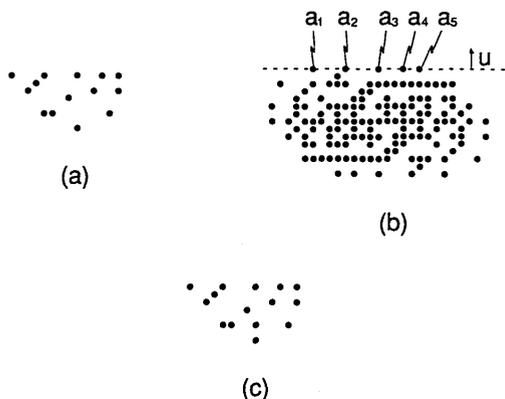
Fig. 7. Example of the totally asymmetric rule. (a) Set  $S$  consisting of discrete points, (b) set  $A = S - S$  and  $E(A, u) = \{a_1, a_2, a_3, a_4, a_5\}$ , (c) a single-sided locator set  $L = A \cap [\cap_1^5 (A + a_i)]$  determined by the asymmetric rule. Note that  $L$  is the same as a translation of the original support  $S$  except for one extra point.
