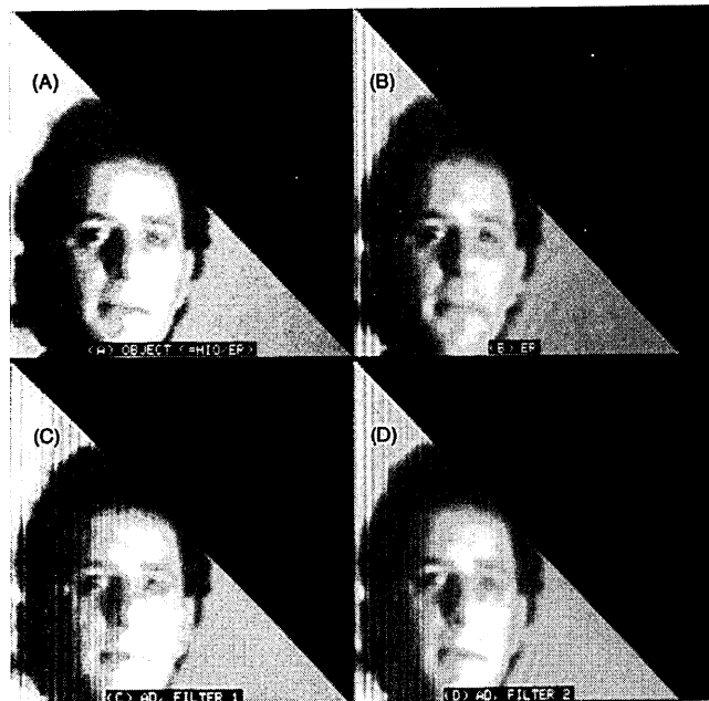
Fig. 3. Comparison of phase-retrieval using AD blind deconvolution with the HIO and ER iterative transform algorithms for a real-valued, nonnegative object with known support and no Fourier modulus error. Reconstructed images: (A) HIO/ER (indistinguishable from the original object); (B) ER; (C) AD with the Fourier constraint of Eq. (14); (D) AD with the Fourier constraint of Eq. (15).
