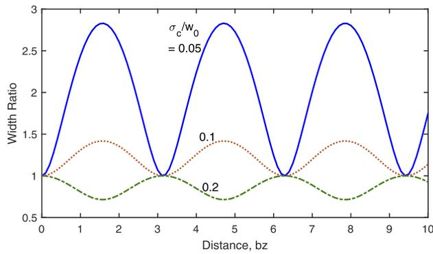
**Fig. 1.** Variations in the width of a partially coherent beam plotted as a function of  $bz$  for three values of the ratio  $\sigma_c/w_0$ .
