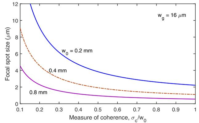
**Fig. 2.** Focal spot size of a partially coherent beam plotted as a function of  $\sigma_c/w_0$  for three values of the beam's initial width.
