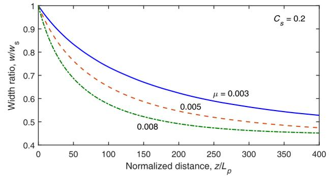
**Fig. 2.** Predicted decrease in the width of the signal beam as a function of  $z/L_p$  for three values of  $\mu$ .
