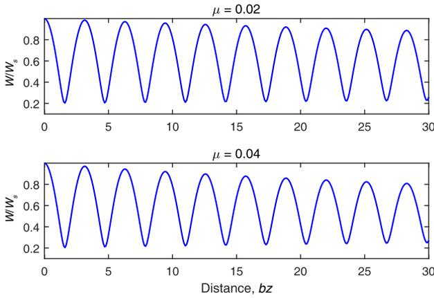
**Fig. 1.** Oscillations in the width of the signal beam for two values of the parameter  $\mu$ . The amplitude of oscillations does not change when  $\mu = 0$ .
