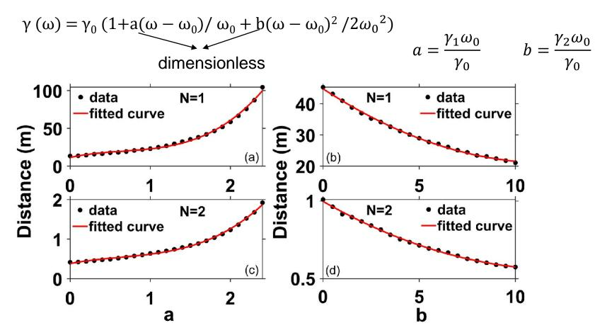
The length scale is reduced by a factor of 50 when we switch from N=1 to N=2 soliton
