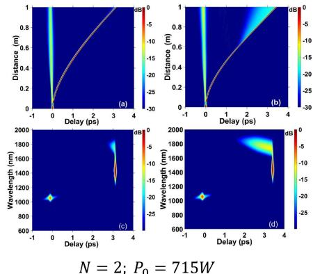
Additional spectral feature at 1620 nm due to the trapping of the NSR
