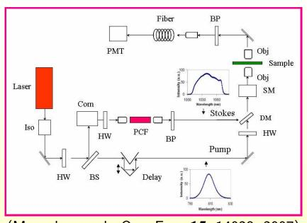
(Murugkar et al., Opt. Exp. **15**, 14028, 2007) Laser pulses (65-fs) split to produce pump and Stokes beams. Bandpass filter after the PCF selects the Stokes bandwidth. Different Stokes frequencies excite different molecules in sample.
