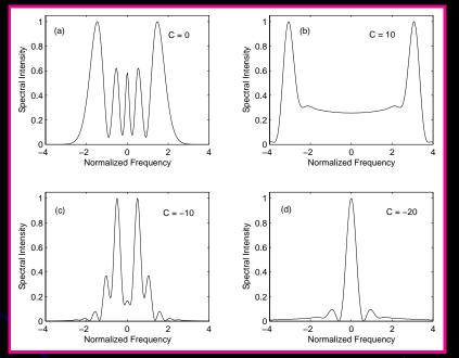
• Chirped Gaussian pulses with  $A(0,t) = A_0 \exp[-\frac{1}{2}(1+iC)(t/T_0)^2]$ .
