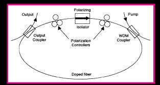
• Different nonlinear phase shifts for the two polarization components: nonlinear polarization rotation.
