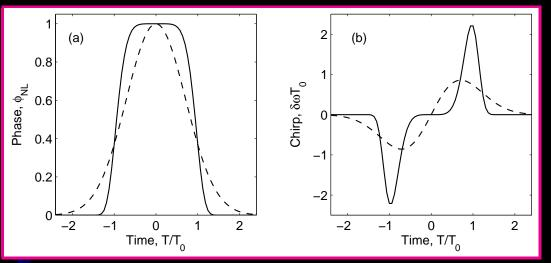
• Super-Gaussian pulses:  $P(t) = P_0 \exp[-(t/T)^{2m}]$ .
