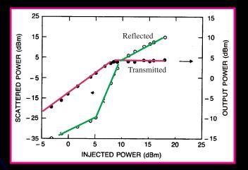
Most of the power reflected backward after SBS threshold is reached.
