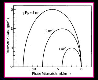
In the case of a single pump:  $g(\boldsymbol{\omega}) = \sqrt{(\gamma P_0)^2 - \kappa^2(\boldsymbol{\omega})/4}.$
