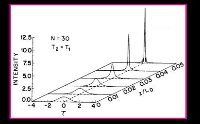
• An intense pump pulse is copropagated with the low-energy pulse requiring compression.
