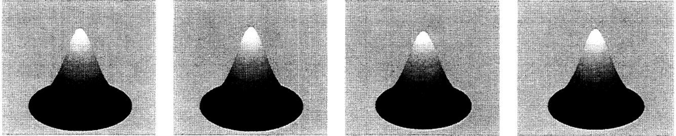
Fig. 5. The transverse mode patterns of the light fields from four of the pulses from a current modulation at 2.5 GHz with  $J_{ac}/J_{dc} = 0.5$
