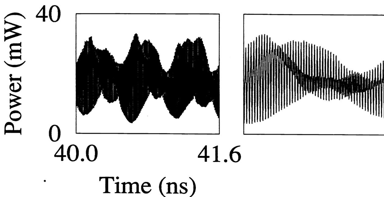
Figure 6. FM wave emitted by three-mode laser operating at 60% above threshold and  $\kappa\tau = 4$ . A close-up version of 0.5 ns is also shown.
