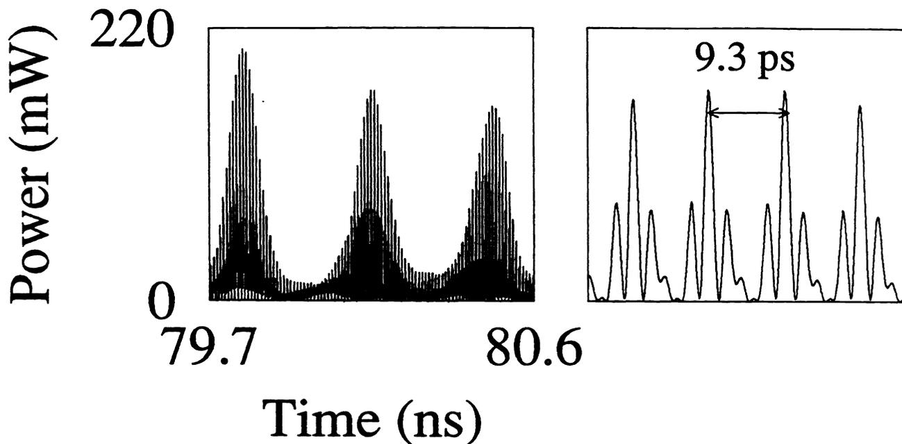
Figure 4. Mode locked pulse train (a) and individual pulses (b) for a six-mode laser operating at 60% above threshold and  $\kappa\tau = 4.9$ .
