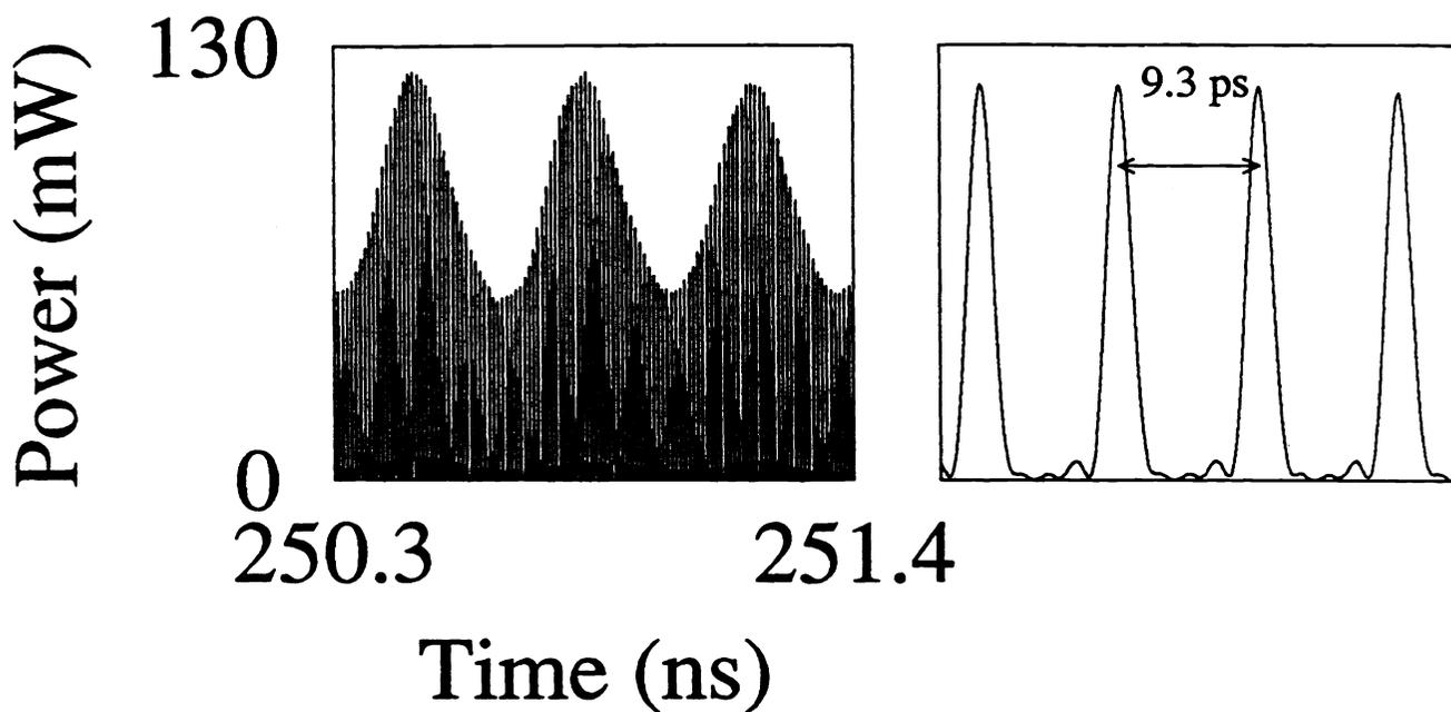
Figure 3. Mode locked pulse train (a) and individual pulses (b) for a five-mode laser operating at 60% above threshold and  $\kappa\tau = 1.0$ .
