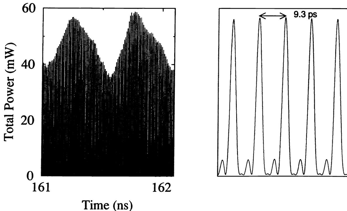
Figure 2. (a) Representative mode-locked pulse train for  $\kappa\tau = 2.0$ . The intensity modulation is discussed in the text. (b) A zoomed-in version reveals the spacing between pulses as well as the secondary pulse structure.
