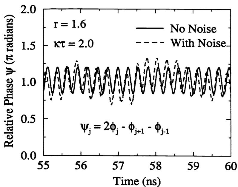
Figure 5. Reduced phase with noise (-----) and without noise (——) for three-mode laser operating at 60% above threshold and  $\kappa\tau = 2$ .
