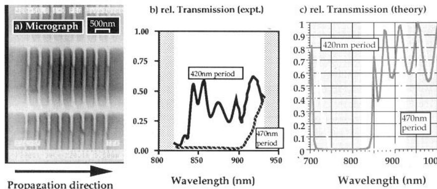
**Figure 1.** Experimental results of a third order 1-D PBG structure and comparison with simulation. (a) Physical structure, 420 nm period, 100 nm airgaps, etched 0.9 µm deep. (b) Normalized transmission through two different waveguide structures (420 and 470 nm period) measured with a tunable Ti:sapphire laser. (c) Simulation of the properties of the same structure. The wavelength range accessible in the measurement is highlighted.
