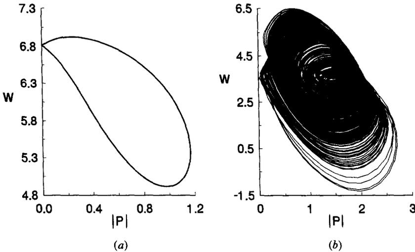
Figure 2. Effect of  $\varepsilon$  on the laser instabilities at the threshold value  $r_{th} = 7$ . (a)  $\varepsilon = 0$  and (b)  $\varepsilon = 0.4$ . All parameters are scaled in terms of  $\gamma_T$ .
