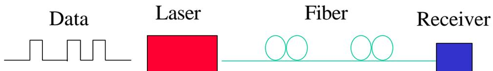
Figure 1.2: Basic elements of a fiber-optic communication system
