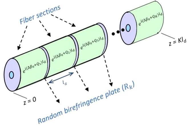
Fig. 1. Model used for calculating the random linear transfer matrix  $\mathbf{T}$ . The fiber is divided into  $K$  sections of length  $l_d$ , and each section is followed by a random birefringence plate.
