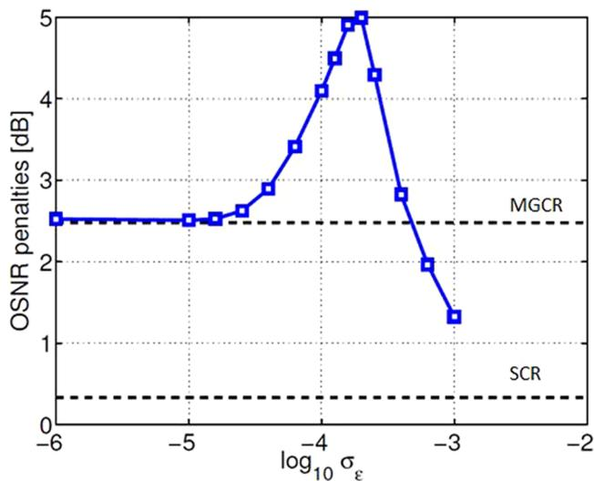
Fig. 3. OSNR penalties for a 6 channel SDM system, transmitted over 1000 km 28.5-Gbaud channels in the QPSK format, as a function of  $\sigma_\epsilon$ . The dashed horizontal lines show the penalties obtained by using the averaged equations.
