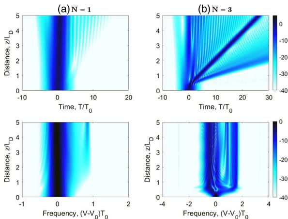
**Fig. 4.** Effect of TOD on soliton evolution for (a)  $\tilde{N} = 1$  and (b)  $\tilde{N} = 3$  for the parameter values used in Fig. 1(a).
