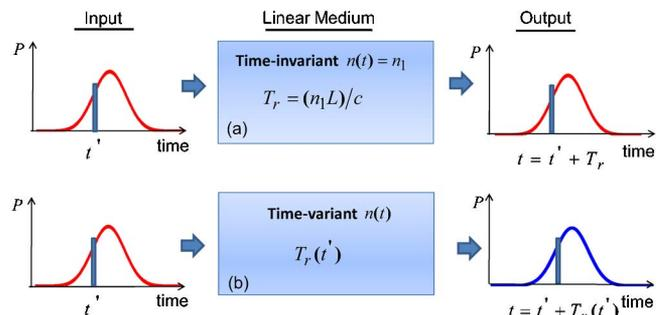
Fig. 1. (Color online) Input and output pulses of linear systems: (a) time-invariant and (b) time-variant medium. Each temporal slice of input pulse is delayed by a transit time  $T_r$ , which is constant for the time-invariant case, but time dependent for the time-variant case.
