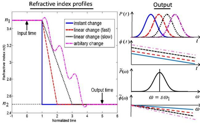
Fig. 3. (Color online) Four dynamic refractive index profiles and the corresponding output pulses. In all cases, the refractive index is initially  $n_1$  and becomes  $n_2$  after the change. The output pulses are identical in temporal shape and spectral power, but have different time delays.
