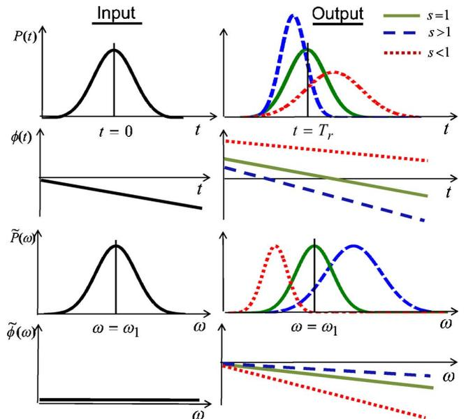
Fig. 2. (Color online) Input (left column) and output (right column) traces showing the power and phase profiles of Gaussian pulses in the temporal and spectral domains. The dashed (blue), solid (green), and dotted (red) curves correspond to stretching factors of  $s = 3/2$ , 1, and  $2/3$ , respectively. We choose a linear variation of  $n(\tau)$  for  $s \neq 1$ , while preserving the interval  $T_f - T_i = 0.5n_1 L/c$ .
