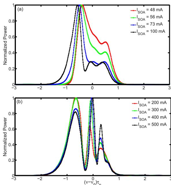
Fig. 2. (Color online) Observed spectra of amplified pulses at drive current (a) up to 100 mA and (b) beyond 100 mA.
