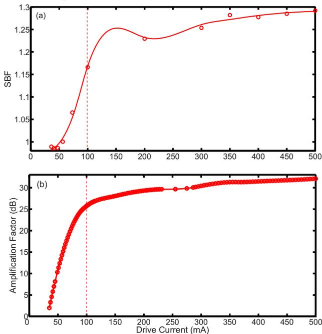
Fig. 4. (Color online) (a) Spectral broadening factor (SBF) and (b) measured small-signal amplification factor as a function of drive current.
