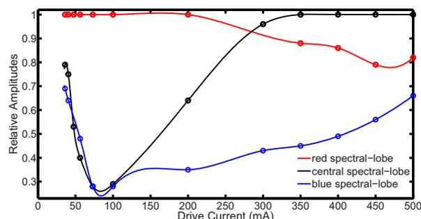
Fig. 3. (Color online) Relative amplitudes of the three main spectral lobes seen in Fig. 2 as a function of drive current.
