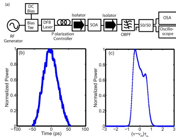
Fig. 1. (Color online) (a) Experimental setup. (b) Pulse shape and (c) pulse spectrum produced by the gain-switched DFB laser.
