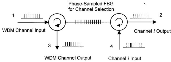
Fig. 1. Schematic of an ADM designed for broad-band dispersion compensation. It consists of two three-port optical circulators and one purely phase-sampled FBG.
