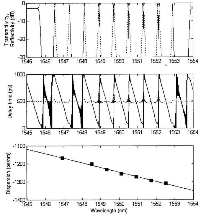
Fig. 3. Transmittivity (dotted line) and reflectivity (solid line) for the phase profile of Fig. 2 (top), resulting group delay (middle), and dispersion  $D$  at the WDM channel wavelength (bottom) for the ADM designed to drop a single WDM channel.
