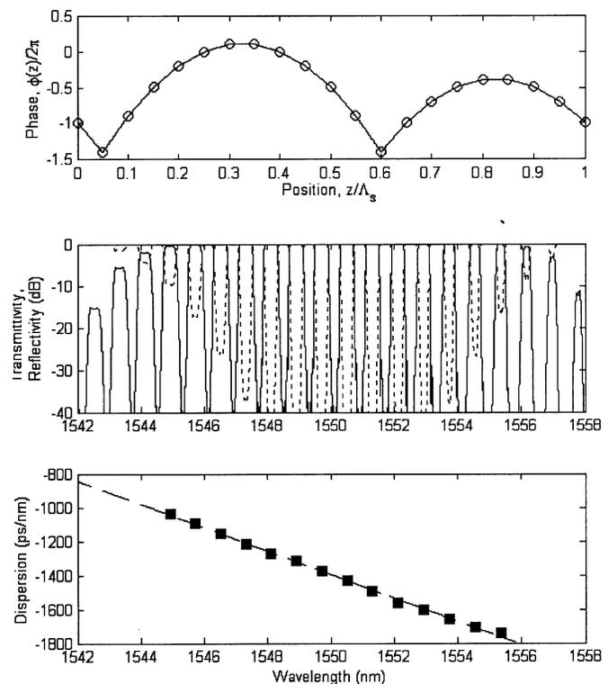
Fig. 5. Same as in Fig. 4 except that the phase-sampled grating is designed to act as a channel interleaver by dropping or adding alternate channels.
