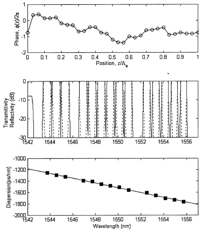
Fig. 4. Optimized phase profile an ADM designed drop (and add) Channels 4 and 11 among the 16 WDM channels. Transmittivity and reflectivity spectra (middle) and dispersion  $D$  at the WDM channel wavelength (bottom) are also shown for such a multichannel ADM.
