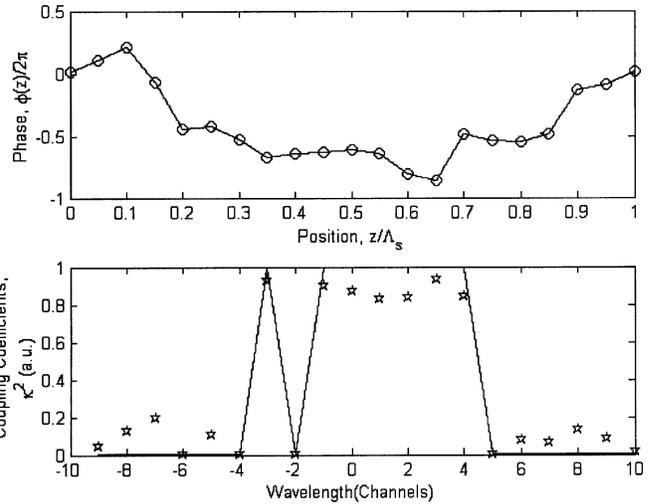
Fig. 2. Optimized phase profile of the ADM designed to drop (and add) Channel 2 in an eight-channel WDM signal. Resulting coupling coefficient is shown in the bottom panel. Stars denote the location of wavelength channels.
