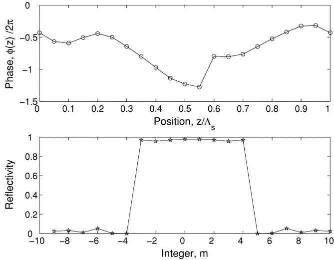
Fig. 2. Optimized phase profile for each sample (top) and resulting reflectivity spectrum (bottom). Stars denote the location of wavelength channels.
