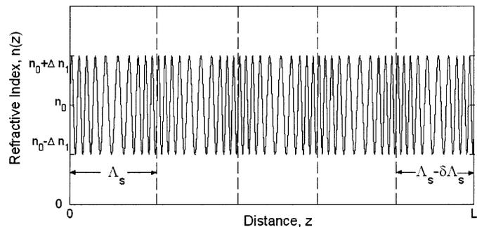
Fig. 1. Schematics of a purely phase-sampled Bragg grating. The sampling period  $\Lambda_s$  is chirped such that it is reduced by  $\delta\Lambda_s$  at the end of grating.
