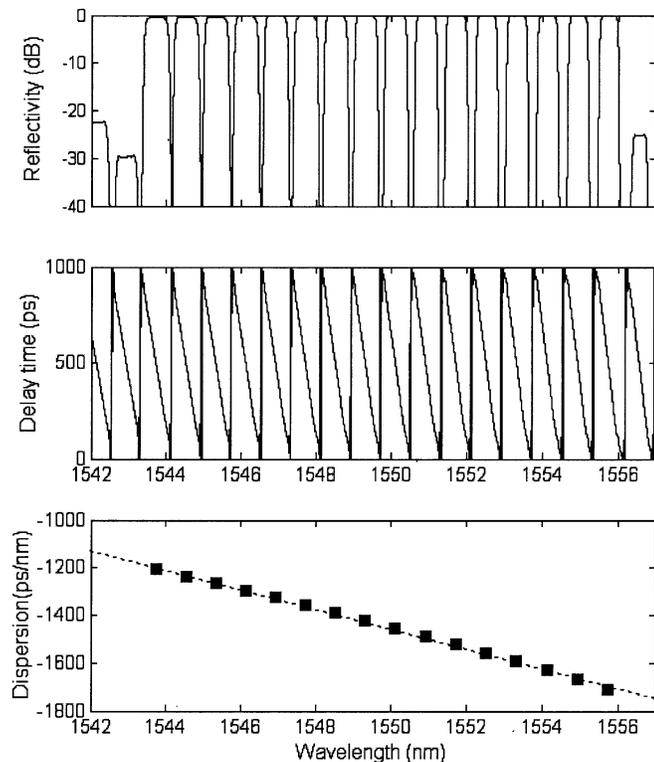
Fig. 5. Reflectivity, group delay, and dispersion of a phase-sampled grating designed for 16 WDM channels. The sampling period is chirped such that it is reduced by 2.1% over the grating length.
