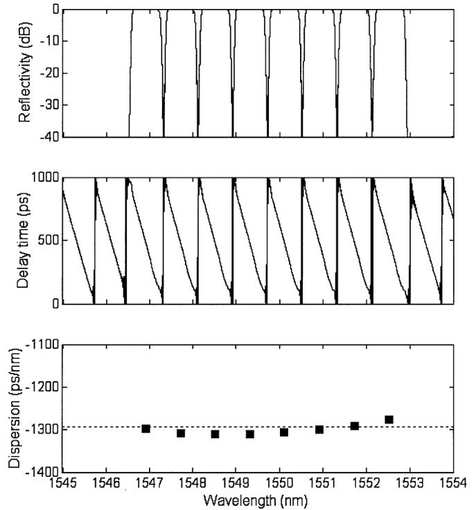
Fig. 3. Reflectivity, group delay, and dispersion of a phase-sampled FBG designed for eight WDM channels. The grating period is chirped but the sampling period is constant.
