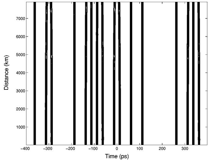
Fig. 3. Contour map of the bit sequence over 8000 km for the 40-Gb/s system employing lumped amplifiers with 100-km amplifier spacing.
