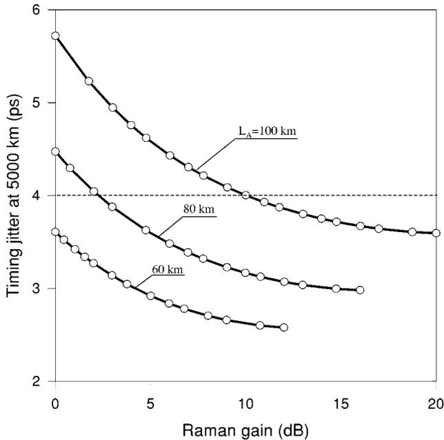
Fig. 2. Timing jitter after 5000 km as a function of Raman gain for amplifier spacings of 60, 80, and 100 km.
