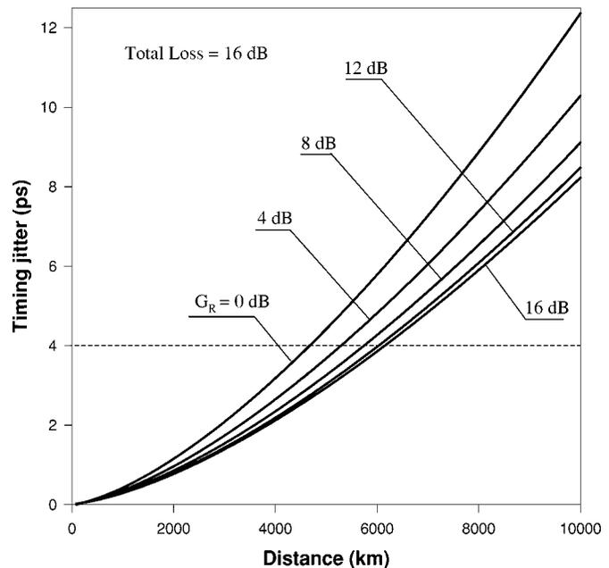
Fig. 1. Timing jitter after each amplifier as a function of transmission distance for several values of Raman gain. Losses are 16 dB over 80 km of amplifier spacing.
