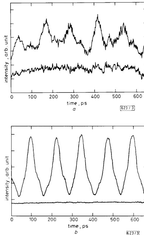
Fig. 3 Streak camera recording of 16 Gbit/s, 0101 ... pulse train after 70 km of fibre and without dispersion compensation
