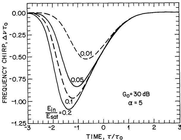
Fig. 1. Frequency-chirp profiles of the amplified pulse for several input pulse energies when a Gaussian pulse is amplified in a semiconductor-laser amplifier with an unsaturated gain of 30 dB.
