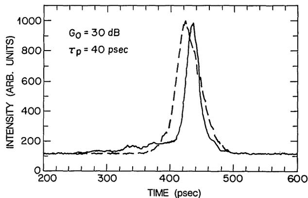
Fig. 3. Experimental traces of the pulse shape obtained by using a streak camera for the compressed pulse (solid curve) and the input pulse (dashed curve).
