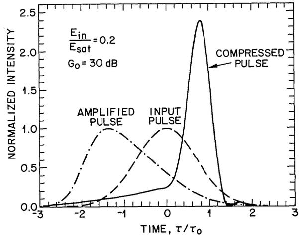
Fig. 2. Compressed pulse when the amplified pulse is passed through a dispersive delay line such that  $L_C/L_D = 0.3$ . The dashed curve shows the input pulse, and the dotted-dashed curve shows the amplified pulse before compression.
