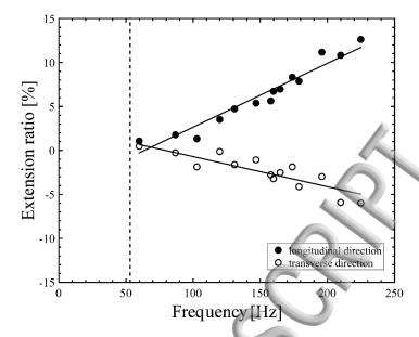
Figure 3: Variation of the extension ratios for the superhydrophobic PDMS surface as a function of natural frequency of the surface. The solid lines are linear square fits to the data. The dotted line indicates the frequency for the surface without tension.
